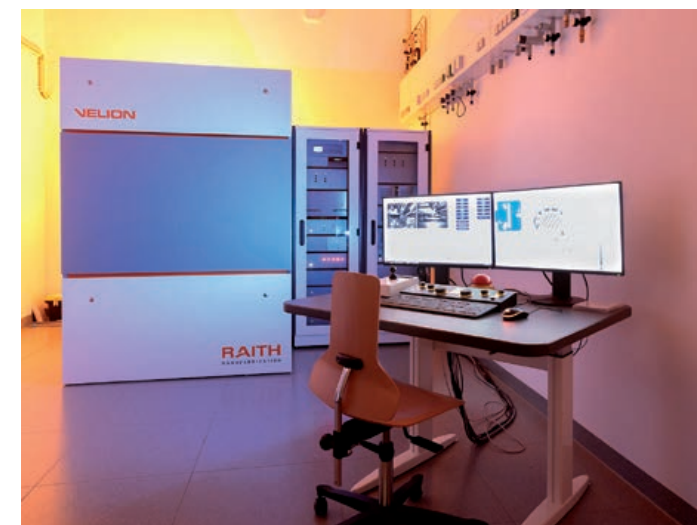
Das neue Ionenstrahlolithografie-System im Center for Soft Nanoscience The new ion-beam lithography system at the Center for Soft Nanoscience
